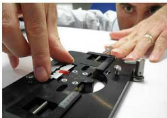
Step 3. Cross-section sample with razor.
