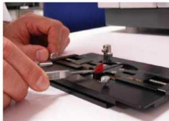
Step 2. Place sample into micro-vice.
