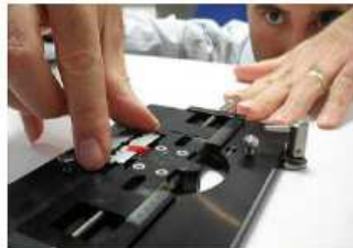
Step 3. Cross-section sample with razor.
