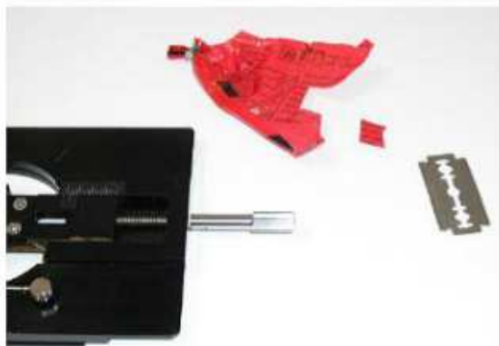
Step 1. Cut a small piece of sample.
