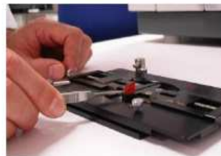
Step 2. Place sample into micro-vice.
