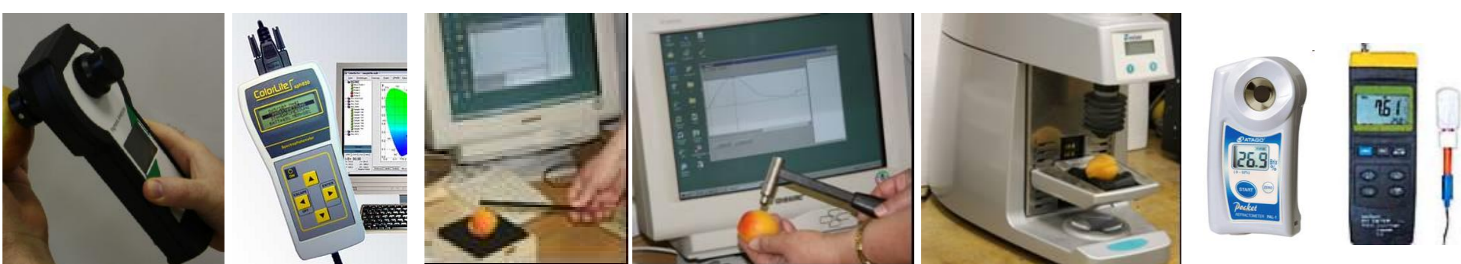
Fig. 3: Pigment Analyzer, Color Lite; Acoustic method, Impact method, Sinclair IQ tester; Brix tester, pH-meter
